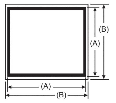
ALL MEASUREMENTS OF BOX FRAME SCREENS ARE (A) BOX TO BOX. YOU MUST <u>SPECIFY</u> (A) MEASUREMENT BOX TO BOX WHEN ORDERING FLANGED SCREENS.
