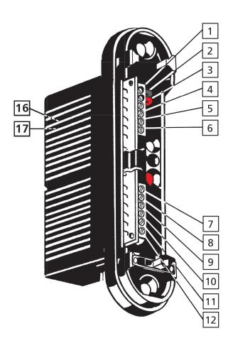
The FUHR multitronic control unit is equipped with a multitude of input and output sockets to connect additional components (such as e.g. transponder, eye scan, finger print, code locks, electrical swing door opener, alarm systems, facility management systems etc.). The input and output sockets are located:
