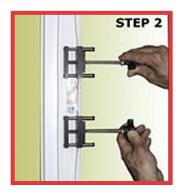
2. Turn knobs clockwise by hand or with a hex bit drill gun to spread jamb.
