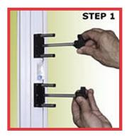
1. Position one spreader below and one spreader above the item needing removal.
