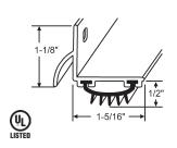
900-14246 36" Long. Mill. For 1-3/8" or 1-3/4" Doors. Includes Fasteners.
