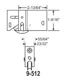
Steel Outer & Inner Housing with 1-1/2" Steel Wheel PGT
