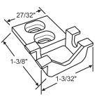
900-5987 Nylon Sliding Roller Housing. Used with 900-10015 Roller
