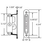
900-18867 Diagonal Hub. Aluminum Finish Use: 900-14560 for Keeper TRACO
