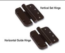
Engineered for maximum strength and security, Sentry Hinges exceed ANSI grade 3 requirements for doors weighing up to 220 lbs. Sentry Hinges exceed ANSI grade 1 impact specifications. Sentry Hinges are made of extruded brass and extruded aluminum that provides superior strength and corrosion resistance. Sentry Hinges provided with non-removable pins for maximum security.
