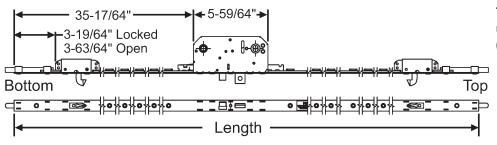
The 5-point active lock mechanism is used on double active Stormwatch™ (AP/PA) units.
