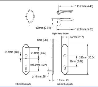
**Brushed Chrome Resista®** Type Material **Rustic Umber** Active Door Set - 90° Cylinder Solid Brass 850-2427235 850-2427340 Active Door Set - Cylinder Not Included Solid Brass 850-2427382 850-2427489 Inactive Door Set - 90° Thumb Turn Insert Solid Brass 850-2427500 850-2427585 Inactive Door Set - Thumb Turn Insert Not Included Solid Brass 850-2427614 850-2427729 Pair Fixed Dummy Solid Brass 850-2427745 850-2427825
