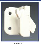
Our 50-2008 series is a single action WOCD designed to install directly to the window jamb extension or return and interact with the active sash of any hung or sliding window. This device comes with mounting hardware to assure proper installation and is available in right & left handing. The 50-2008 series was designed to be applied in the field or in the factory.
